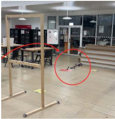
Fig. 61: Flight test obstacle: The drone is successfully traversing a window sized opening whose shape is smaller than the UAV's full wingspan.
