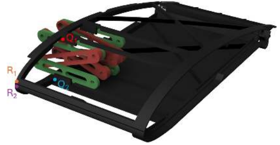
Fig. 12: position of points Q (attachment point between the link and the wing surface) and R (inner tip of the leading edge)
